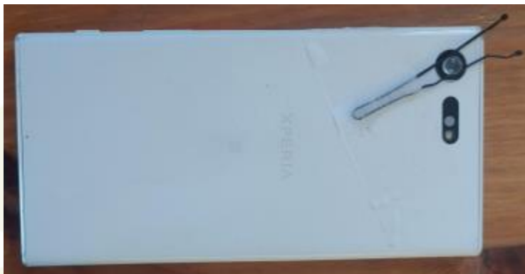
Photo: A lens attached to a smartphone camera using a hairpin and adhesive tape. (Photo: Sara Gorenjak)
