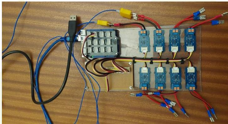
Figure 2 – Arduino-based data logger.
