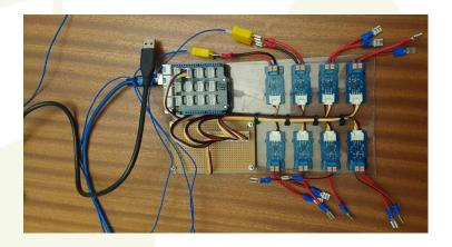
Figure 2 – Arduino-based data logger.
