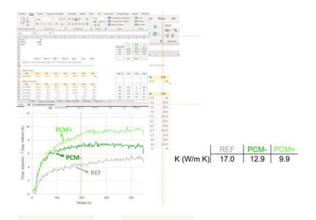
Figure 3 – Example of the datasheet showing the collected data, graphical representation, and thermal conductivity results of the building material samples.
