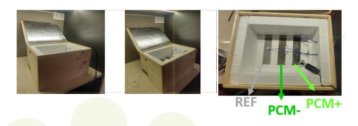
Figure 1 - Setup for measuring thermal conductivity
