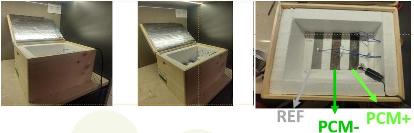
Figure 1 - Setup for measuring thermal conductivity
